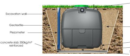
Top fill = see height indicated on the product's data sheet (sand + max. 20 cm of topsoil)
