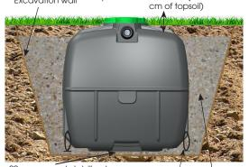
20 cm cement-stabilized sand bed 200ka/m<sup>3</sup> + reinforced welded mesh
