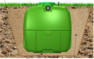
10 cm bed of compacted sand or rolled gravel 2/4 mm
