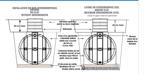
tank, create a self-supporting reinforced concrete slab supported on stabilized, undisturbed ground all around the excavation in the following cases:
