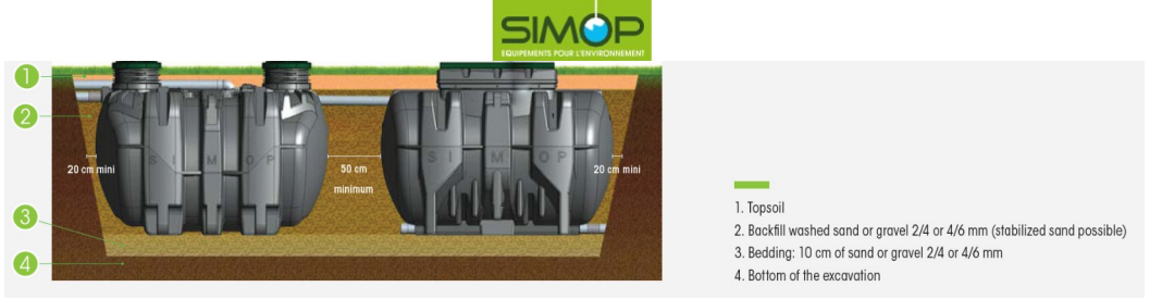
Figure 19: Cross-section of the installation in normal terrain
